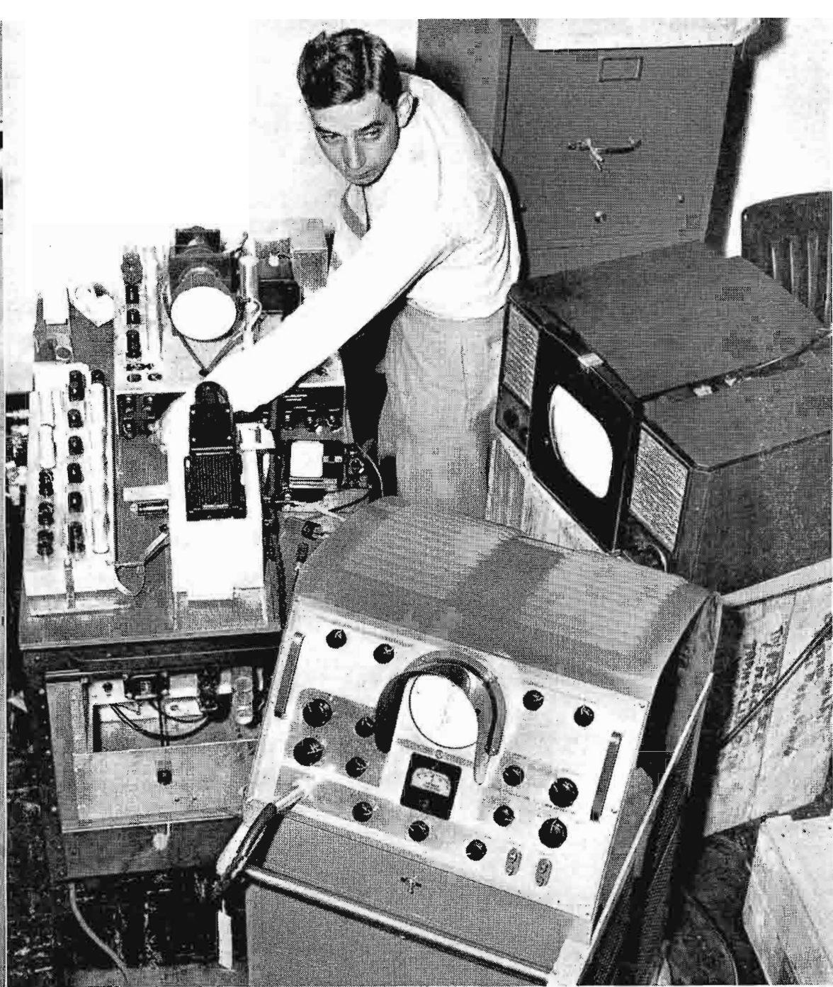
FIG. 7. Lining up the flying spot generator built by NBC engineers for use in generating test patterns.
