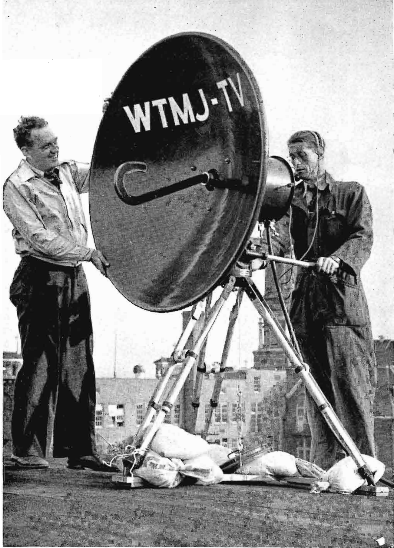
FIG. 1. WTMJ-TV's new television equipment includes complete RCA Microwave Equipment for relaying remote programs to the studio.
