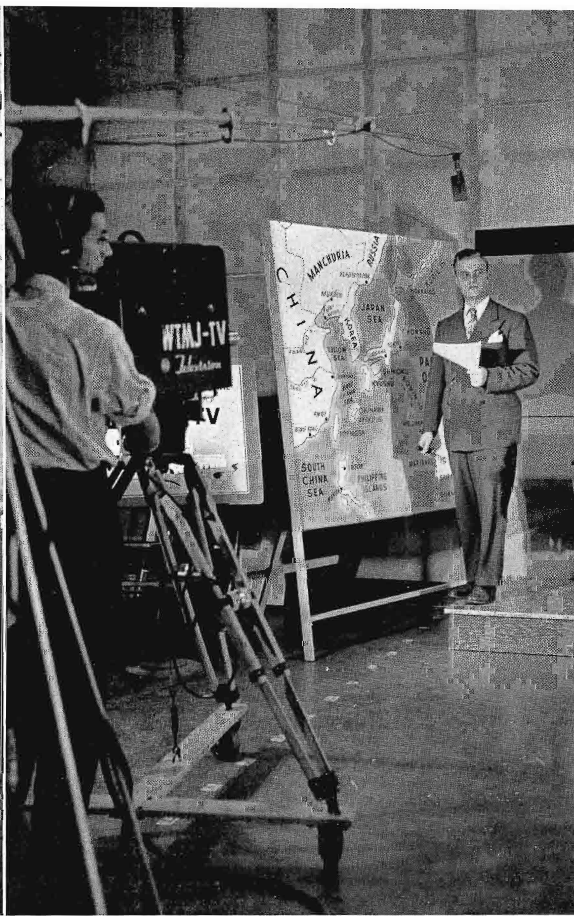
FIG. 2. Two image-orthicon field camera chains are included in WTMJ-TV's equipment. At present these are used for both studio and field use. Additional cameras which have been ordered will be installed for permanent studio use.
