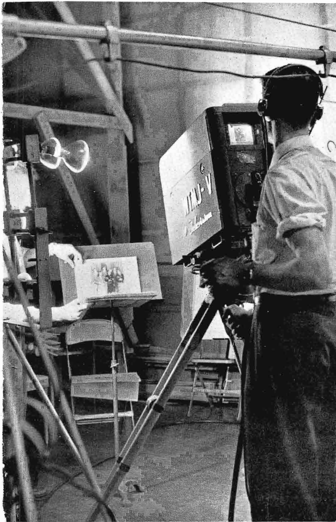
FIG. 2. Two image-orthicon field camera chains are included in WTMJ-TV's equipment. At present these are used for both studio and field use. Additional cameras which have been ordered will be installed for permanent studio use.
