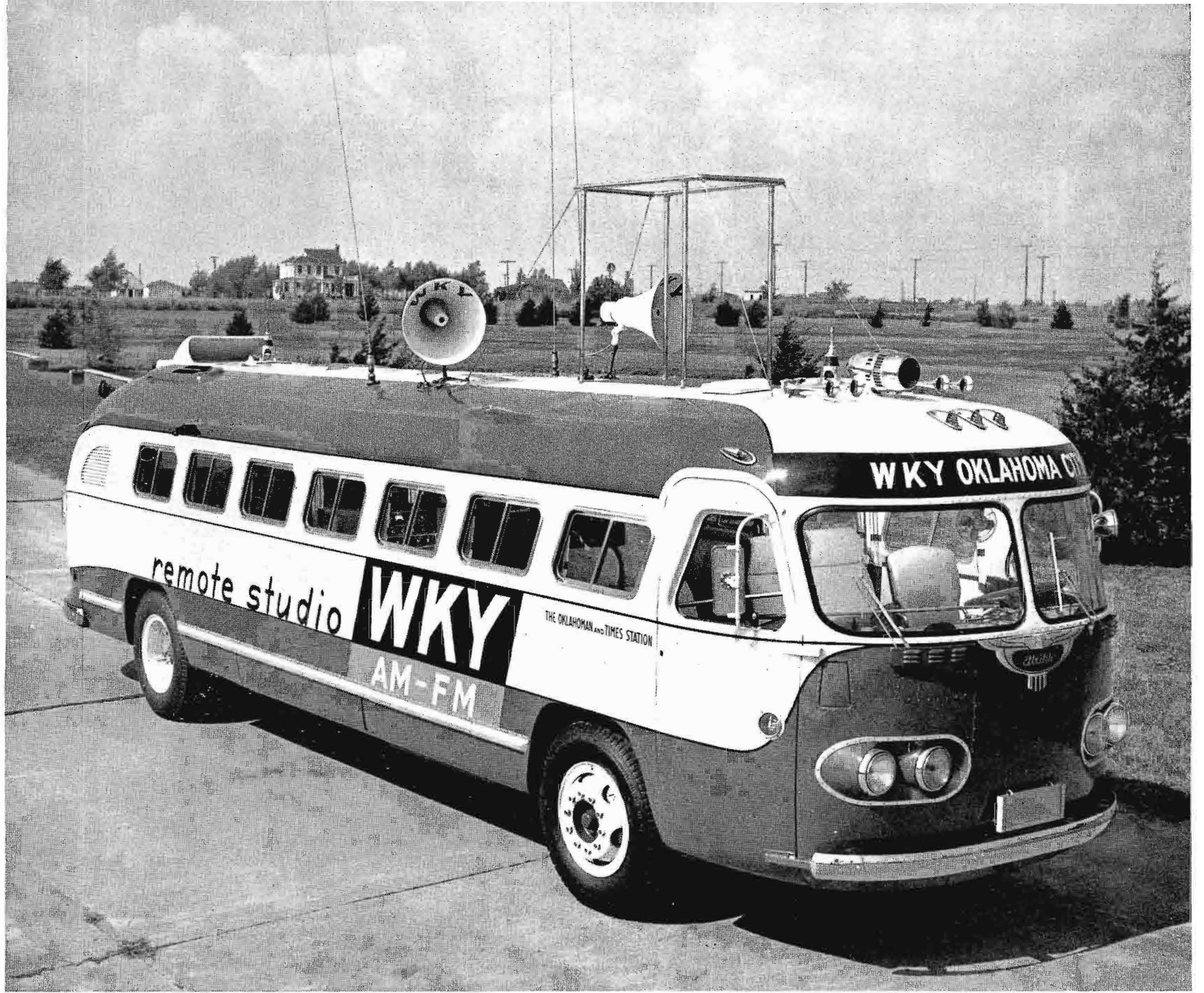
FIG. 1. WKY's mobile unit—built to permit coverage of an entire state—is a 29 passenger bus body, custom-converted by the bus manufacturer according to plans drawn by WKY's engineering staff. Complete facilities and comfort for traveling are outstanding features.
