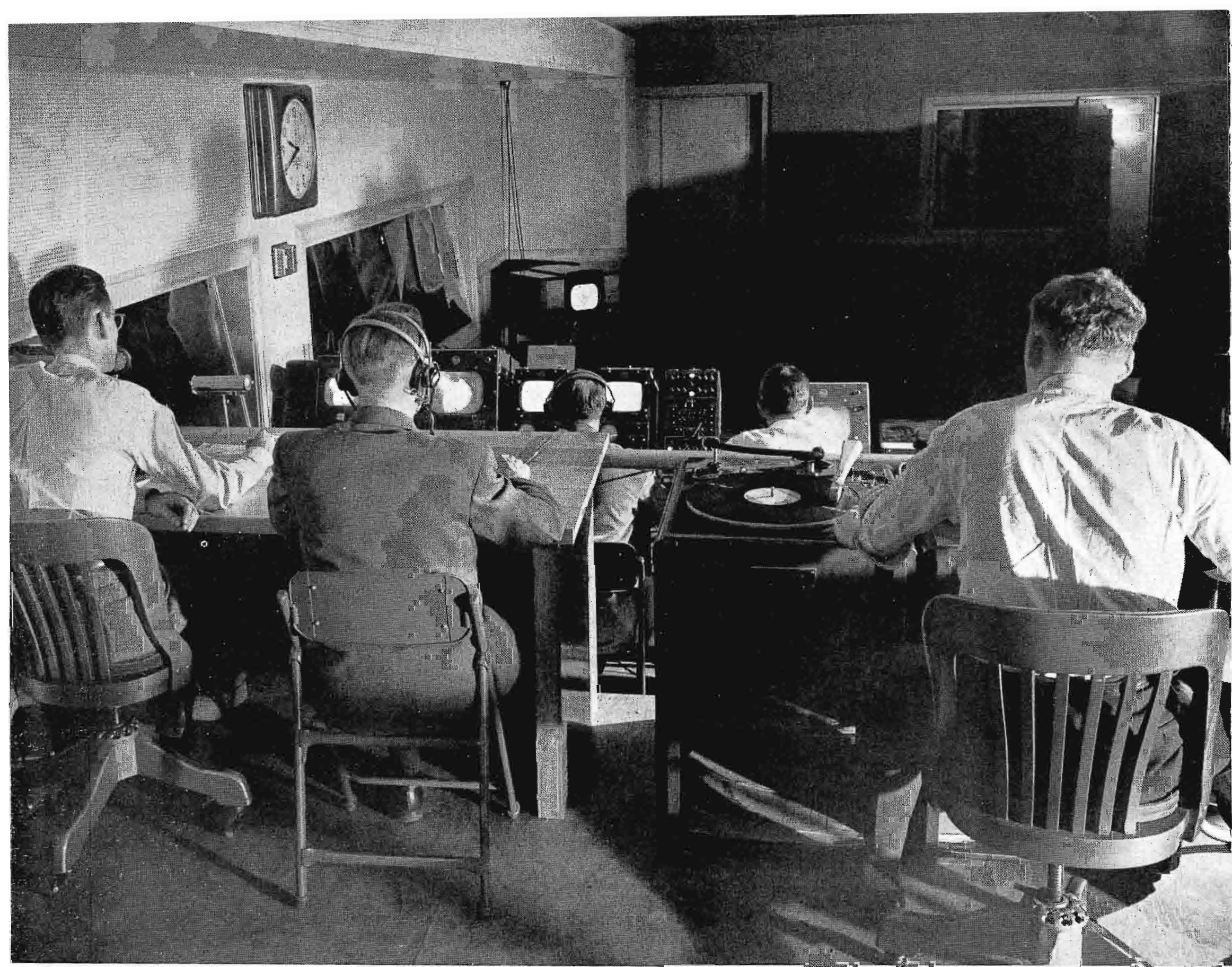
FIG. 3. WTMJ-TV's studio control room. Video operators sit at camera controls on lower level. On upper tier are program director (left), technical director (center) and audio operator (right). The program director has a good view of the studio through the window at his left.
