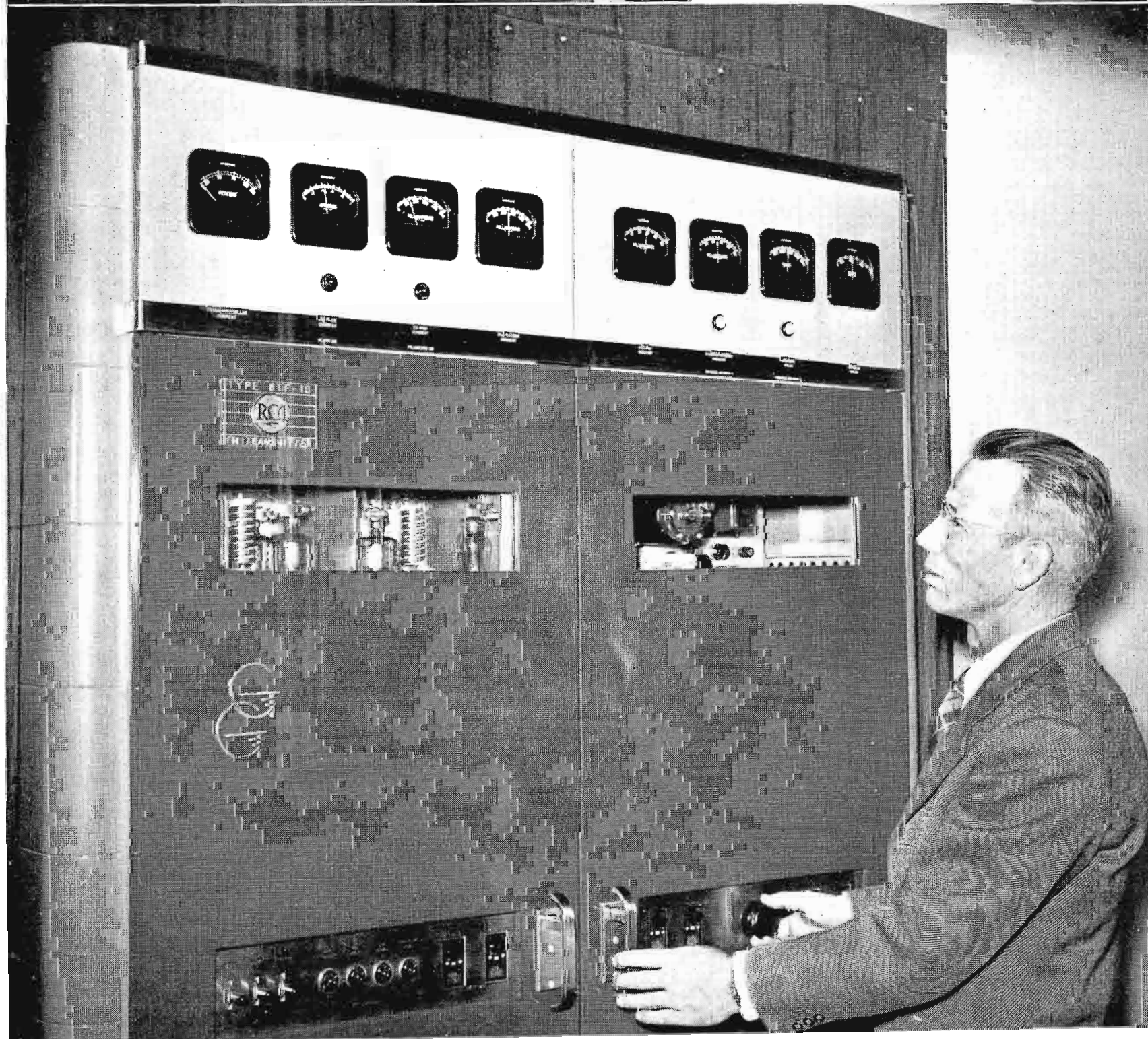
FIG. 4. KFBK's RCA Type BTF-1C FM Transmitter is installed in a separate glass-enclosed room just off of the master control room. In the closeup view shown at the right, Stan Sronce, Chief Engineer of KFBK, is making the final adjustments.
